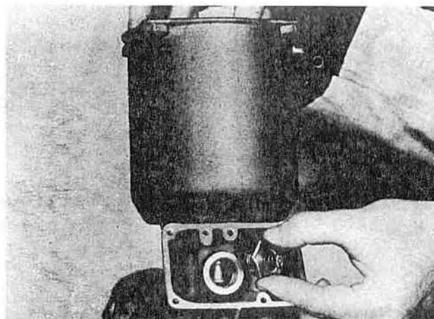
Figure 51—Installing the Compensator Port and Valve
