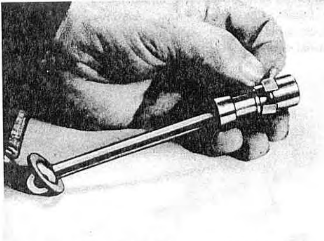
Figure 30—Removing Vacuum Valve Screen
