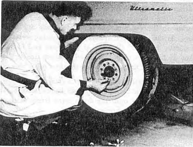
Figure 9—Removing the Rear Wheel from the Hub
