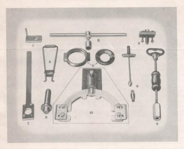
Tools numbered from 1 to 9 inclusive have been previously available to Packard Dealers and are essential for performing rear axle service operations. Each Packard Dealer should check his tool inventory and order tools not on hand. Tool No. 10 (J-3289) is a new tool and is optional for Packard Dealers.
