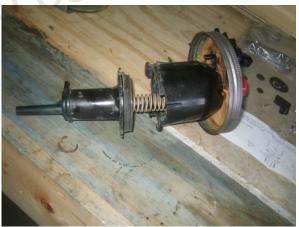
Remove the main spring from the lower half of the pump body. One coil of my spring was rusted off.
