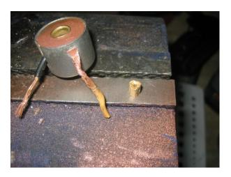
The old frayed wire on my solenoid had a unknown color cloth cover over yellow plastic insulation. I just replaced it with new yellow wire.
