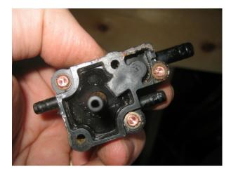
Separate the upper portion of the vacuum control.
