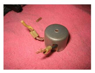
Crush the brass wire crimp in a vise the opposite way of the crimp to open it.
