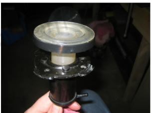
Insert the inner plunger into the outer plunger. Replace the spring with the new spring from the kit.
