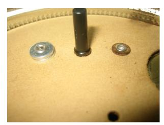
This is what it looks like from the top side. Make sure that the vacuum control is flat and firmly seated against the lid. If there is any play, then seat the rivets more firmly.
