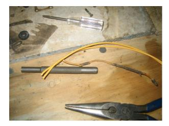
To replace to brass crimps I simply cut the insulation of a blue butt-style connector, to extract the metal interior. I then cut the metal portion in half with a hack-saw, deburring the ends.
