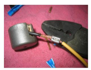
Here both wire have been crimped
