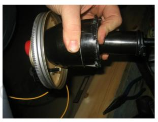
With the retainer in place, both halves should now be locked together.
