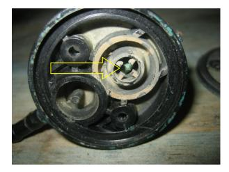
I used a plastic tube from a can of cleaner to push out the screen.
