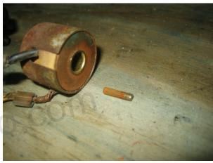
Pull the outer seal up and over the solenoid shaft. Discard the seal. If the seal is hardened, then just break it off.
