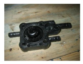
Flip the middle section over, and install the new seal on the end of the button plunger shaft.
