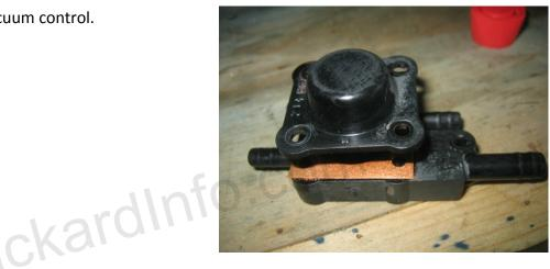
Flip over, and the new rubber valve seal
