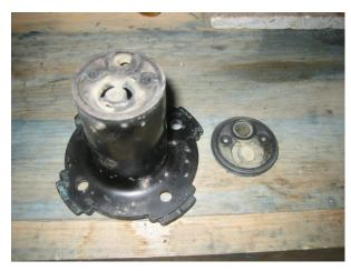
Inside the pick-up portion is a small brass screen. This should be removed and cleaned, or replaced.
