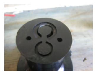
The only instructions included with the rebuild kit was a note to use the included brass screws in attaching the fluid pickup portion to the lower body instead of rivets. To do this you must drill out the rivet holes in the pickup portion (only) with a ¼ drill bit.
