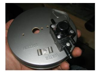
Next the solenoid control was riveted thought the lid and into the upper portion of the pump body. As with the vacuum control, check the solenoid and upper pump body for play. Route the wires under the hold-down.
