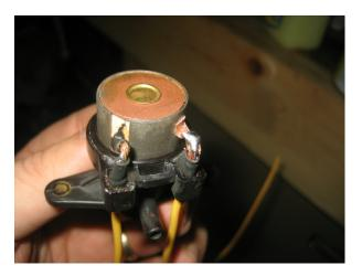
Replace the inner pin, inner spring, and the solenoid plunger.
