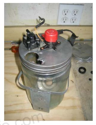
Remove the metal retainer ring that holds the upper and lower section of the pump body together. On my pump this had just disintegrated on me from corrosion.
