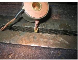
Remove the crimp and separate the remainer of the outer wire from the solenoid wire.
