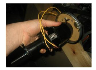
Before the two sections were pushed together, then new retained was slipper over the upper section and pushed down. Now with the two halves together the retainer can be slipped upwards to snap into place.
