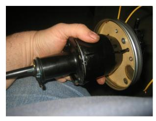
The original wiring was connected to the car harness with bullet-style connectors. To replace these, I simply used new style bullet connectors and removed the blue plastic insulation.
