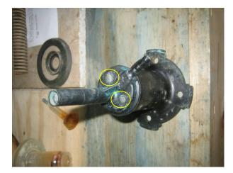
Separate the two pieces, retaining the washers for reuse.
