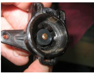
Install the new outer seal on the solenoid shaft
