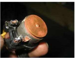
Carefully work the cap down over the solenoid. Adjust and fold the wiring in as needed. Seat the cap evenly and make sure both clips engage the housing.
