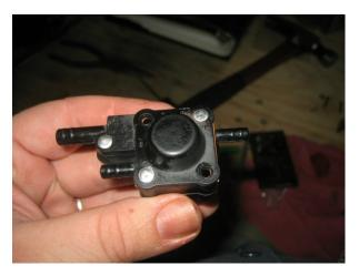
Next install the new inner seal on the solenoid shaft and reinstall into the solenoid body.
