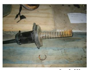
Removed the inner plunger and remover the small spring from the end of it.
