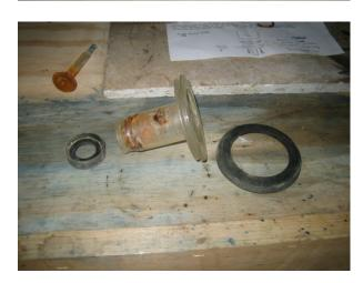
Remove the two rivets that hold the liquid pickup section to the lower pump body. To do this, you need to drill out the peened over area of the rivet from the inside of the pump body. Careful not to drill into the plastic, or the washers under the peened-over portion of the rivets. Use an awl if needed to push the rivets out.
