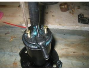
Add the lower seal to the outer plunger.
