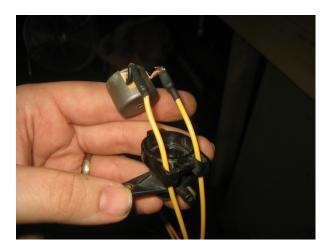
Seat the solenoid into the housing, and push the crimps into their hoses in the housing.
