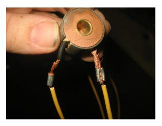
I applied a little solder to each wire as double insurance, and then covered the wire and crimp with heat-shrink tubing to protect it.
