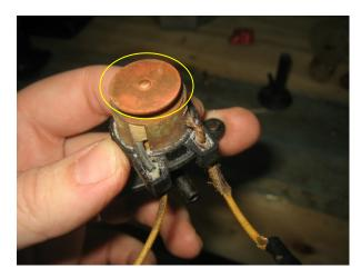
Clip the wires on the outside of housing, leaving the wires inside the housing intact. Gently twist the solenoid side to side to remove it and the brass wire crimps from the housing.
