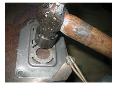
Next the valve body tabs are lined back up with their respective holes in the base plate. Make sure you have the correct orientation of the base-plate to valve body before you do this. With the ends of the valve body resting on the vise, I gently tapped each tab it a crossing pattern until they were all lying flush against the base plate.
