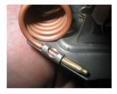
The shaft clip is then reinstalled to link the mechanism back to the valve plunger. I then worked the mechanism lever through it range to make sure there was no binding and the plunger moved in and out freely.
