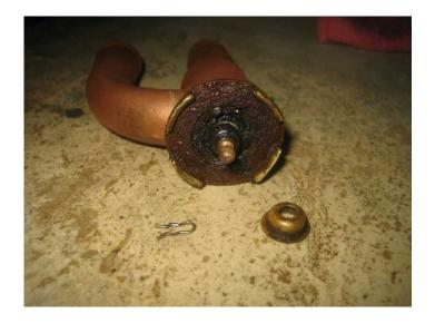
I then removed the plunger from the body, and carefully removed the remains of the old seal.
