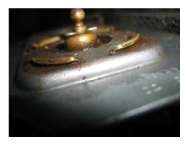
Once the all the tabs were lifted, then I used the blunt edge of a steel ruler, held flat against the base plate, and lightly tapping it with the same small hammer, worked the soft brass tabs vertical. Trying to use pliers at this point would probably just mangle the tabs.
