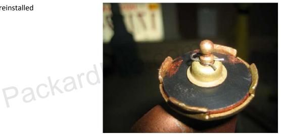
I then sprayed the other side of the seal with a little more copper before the base plate goes back on.
