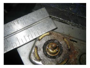
Once all the tabs are vertical, then valve-body should come free from the base plate.
