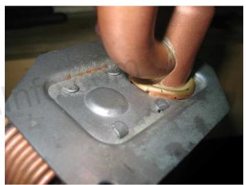
The Thermo-Coil retainer tab is then bent back into place. You want the tab to be tight enough to hold the tube in place firmly, but be careful not to crush the tube.
