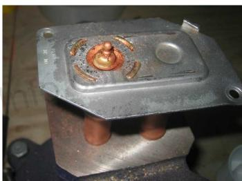
Check the other side of the base plate to make sure that the brass ring is firmly seated all the way around against the base plate.
