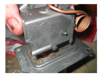
The tabs are then carefully bent flat against the base plate.
