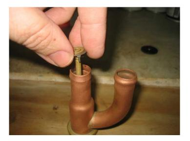
I wiggled the pump body around until the plunger shaft stuck out the hole in the bottom of the valve body. I then inverted the pump body onto a drift held in a vise. This is simply to keep the plunger from falling out while you reinstall the seal, cup, and clip. One note here, the area of the valve body that the seal contacts must be perfectly clean, flat and smooth or it will not seal correctly.
