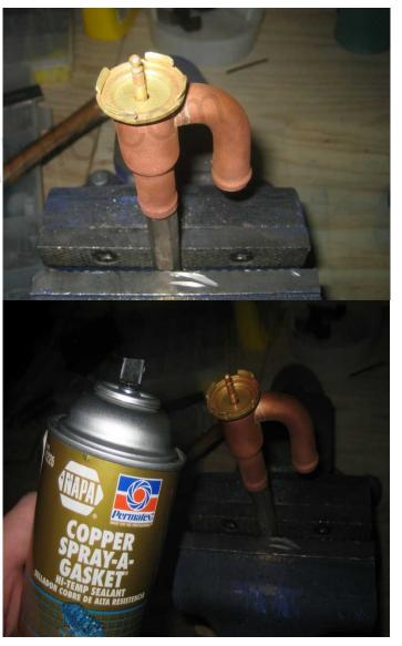
The seal is pushed down over the shaft until firmly seated against the valve body. Make sure the center of the seal is also pushed down far enough to allow the cup to install below the clip groove.
