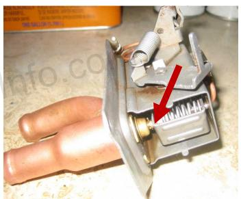
Here in this second picture, the clip has been removed from the shaft, and is just resting on top of it.
